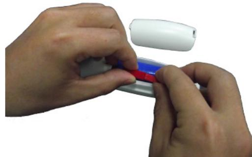
Step 3 : Directly insert the Light Guide into the curing light handpiece. Verify it has been completely inserted into handpiece. Light guide may be rotated to achieve best angle on tooth structure.
